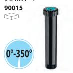
A professional-quality static pop-up sprinkler with an adjustable head from 0° to 350°, that guarantees even irrigation and minimal water consumption (6 l/min). It is equipped with a screw to adjust the jet with a hexagonal insert, stainless steel return spring, filter, self-lubricating clutch and non-spill rubber valve with an anti-freeze device. Ground height of 4" (10 cm).
