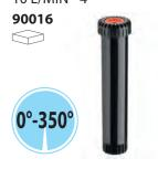
A professional-quality static pop-up sprinkler with an adjustable head from 0° to 350°, that guarantees even irrigation and minimal water consumption (10 l/min). It is equipped with a screw to adjust the jet with a hexagonal insert, stainless steel return spring, filter, self-lubricating clutch and non-spill rubber valve with an anti-freeze device. Ground height of 4" (10 cm).
