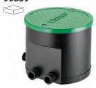
Preassembled valve box incorporating 4 solenoid and a timer. Operates in connection with RF remote control, not included. Power provided by two 1.5V AAA batteries, enough to last an entire season. On/off control for up to 4 independent underground or drip irrigation lines. Easy programming procedure, using just 3 buttons and a large size display. A perfectly sealed IP 68 unit. Wireless connection to radio frequency Rain Sensor.
