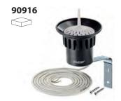
Suitable for all watering systems, the rain sensor avoids unnecessary wastage of water by turning the sprinklers off when it is raining. When the internal flow reaches a level of 5 mm of rain per square metre, the system shuts down. Programmed watering automatically resumes when the water in the sensor evaporates. The rain sensor should be installed in an outdoor area exposed to rain using the stainless steel bracket provided
