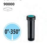
A professional-quality static pop-up sprinkler with an adjustable head from 0° to 350°, that guarantees even irrigation and minimal water consumption (6 l/min). It is equipped with a screw to adjust the jet with a hexagonal insert, stainless steel return spring, filter, self-lubricating clutch and non-spill rubber valve with an anti-freeze device. Height from ground 2" (5 cm).
