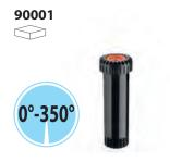
A professional-quality static pop-up sprinkler with an adjustable head from 0° to 350°, that guarantees even irrigation and minimal water consumption (10 l/min). It is equipped with a screw to adjust the jet with a hexagonal insert, stainless steel return spring, filter, self-lubricating clutch and non-spill rubber valve with an anti-freeze device. Height from ground 2" (5 cm).
