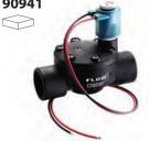
Solenoid with silt filter. Works with the Multipla 9 V timer (cod. 8060) or with the 9 V control unit (cod. 90821). With 1" female inlet and outlet thread. Body in fibre glass reinforced nylon, stainless steel metal components. Low speed shut-off device to prevent pressure shock. Optional manual opening/shut-off control. Operating pressure from 0,5 to 12 bar. Flow rate from 4,6 to 96 l/min. Operating temperature range +5° to +70°.
