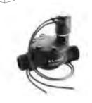
Solenoid with silt filter. Reinforced structure to withstand mechanical and thermal stresses. Operates with all types of multi-line timers at 24 V AC. With 1" male inlet and outlet thread. Body in fibre glass reinforced nylon, stainless steel metal components. Low speed shut-off device to prevent pressure shock. Optional manual opening/shut-off control. Operating pressure from 0,5 to 12 bar. Flow rate from 4,6 to 96 I/ min. Operating temperature range +5° to +70°.
