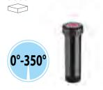
A professional-quality static pop-up sprinkler with an adjustable head from 0° to 350°, that guarantees even irrigation and minimal water consumption (10 l/min). It is equipped with a screw to adjust the jet with a hexagonal insert, stainless steel return spring, filter, self-lubricating clutch and non-spill rubber valve with an anti-freeze device. Height from ground 2" (5 cm).
