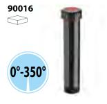
A professional-quality static pop-up sprinkler with an adjustable head from 0° to 350°, that guarantees even irrigation and minimal water consumption (10 l/min). It is equipped with a screw to adjust the jet with a hexagonal insert, stainless steel return spring, filter, self-lubricating clutch and non-spill rubber valve with an anti-freeze device. Ground height of 4" (10 cm).
