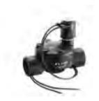
Solenoid with silt filter. Reinforced structure to withstand mechanical and thermal stresses. Operates with all types of multi-line timers at 24 V AC. With 1"female inlet and outlet thread. Body in fibre glass reinforced nylon, stainless steel metal components. Low speed shut-off device to prevent pressure shock. Optional manual opening/shut-off control. Operating pressure from 0,5 to 12 bar. Flow rate from 4,6 to 96 l/min. Operating temperature range  $+5^{\circ}$  to  $+70^{\circ}$ .
